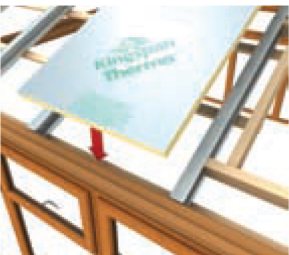
Install external insulation
